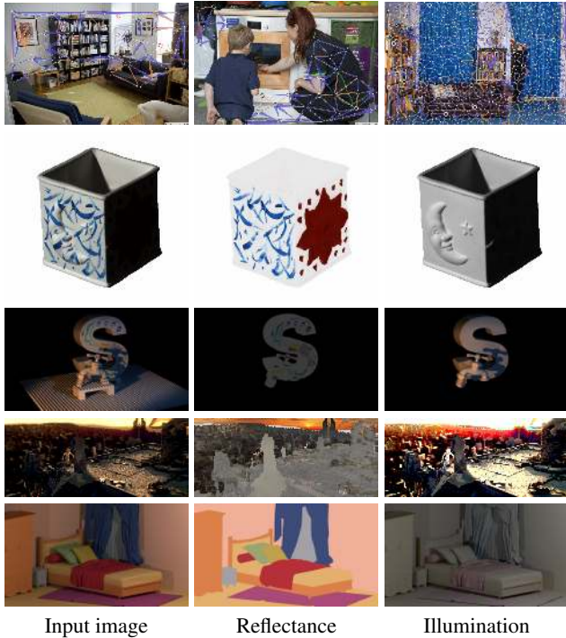
Figure 10: Sample images from existing intrinsic decomposition ground-truth datasets. First row. The database of Bell et al. [BBS14] provides reflectance comparison judgments between pairs of points in photographs of real-world settings (mostly indoor photographs, as illustrated by the overlaid graph). Second row. The MIT database [GJAF09] contains simple isolated objects. Their illumination is obtained by painting the object in white, and the reflectance is obtained by taking the image / illumination ratio. Third row. The MIT database has been extended to more complex scenes by Beigpour et al. [BKK15], exhibiting two objects under various illumination conditions. Fourth row. The Sintel dataset [BWSB12], originally for optical flow evaluation, provides reflectance ground truth videos from synthetic renderings. However, taking the ratio image hardly recovers a valid illumination layer. Fifth row. The database of Beigpour et al. [BSV*13] contains 9 complex but textureless synthetic scenes.
