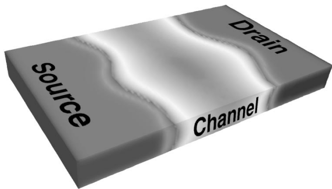
Fig. 10. Potential distribution in a double-gate MOSFET illustrating the effect of LER on the source and drain junctions. LER is defined statistically by its rms amplitude, \Delta , and correlation length, \Lambda .
