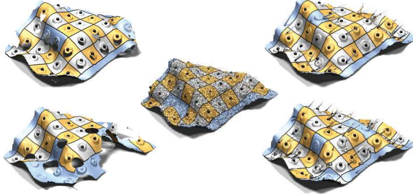
Fig. 6. Robustness of our method to missing and corrupt data: occlusions due to imperfect acquisition and synthetic holes (left), simulated Gaussian noise (center), and shot noise (right). Regions not explained by detected intrinsic structure are in blue.
