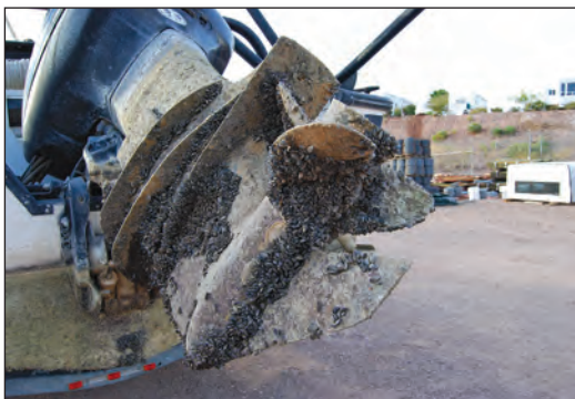
Quagga mussels attached to a boat motor before cleaning. Photograph by National Park Service.
