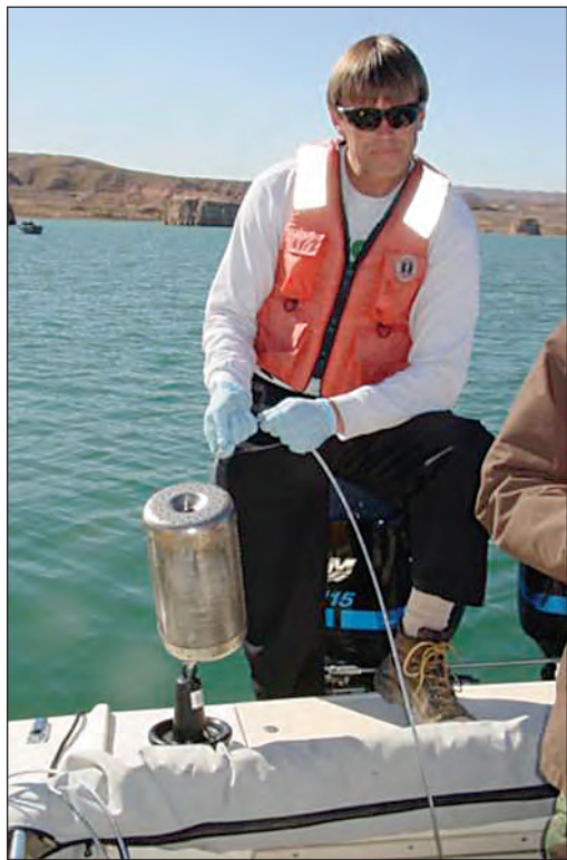
Deployment of SPMD and POCIS containers in Las Vegas Bay for vertical organic contaminant profiling. Photograph by Michael R. Rosen, U.S. Geological Survey.
