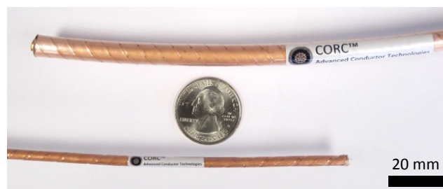
29 30 Figure 1 – 7 mm diameter CORC ® cable (above) made out of 4 mm wide REBCO tapes with 50 \mu\text{m} thick substrates compared to a 31 3.6 mm diameter CORC ® wire (below) made up of 2 mm wide tapes with 30 \mu\text{m} thick substrates.
