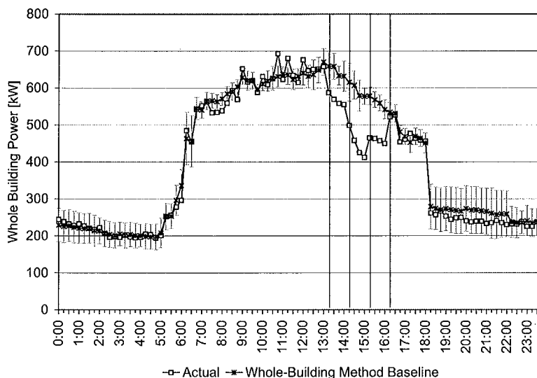
Figure A.9. Total whole building power (fan quantity reduction) - Roche
