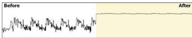
Fig. 20 Balancing power consumption reduces the observed amplitude of data dependant variations (simulated data)
