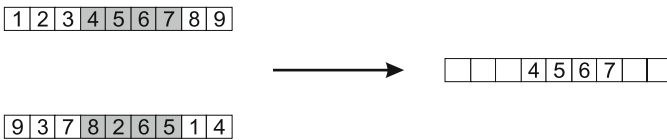
Fig. 4.15. Order crossover, step 1: copy randomly selected segment from first parent into offspring
