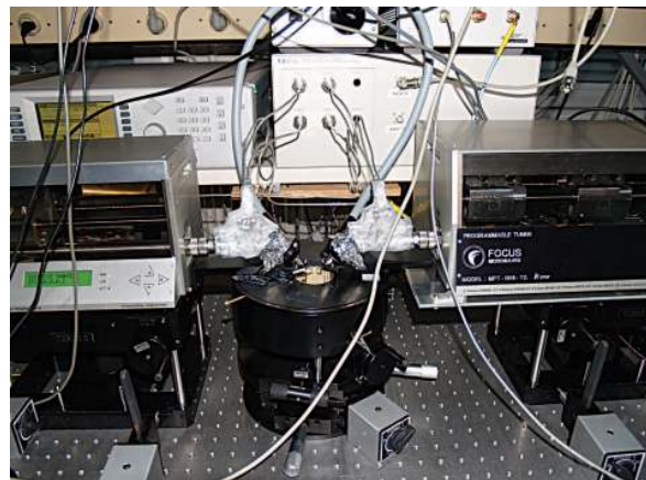
Figure 10. Photograph of a time-domain load-pull system containing wave probes. (Photo courtesy of XLIM, France.)
