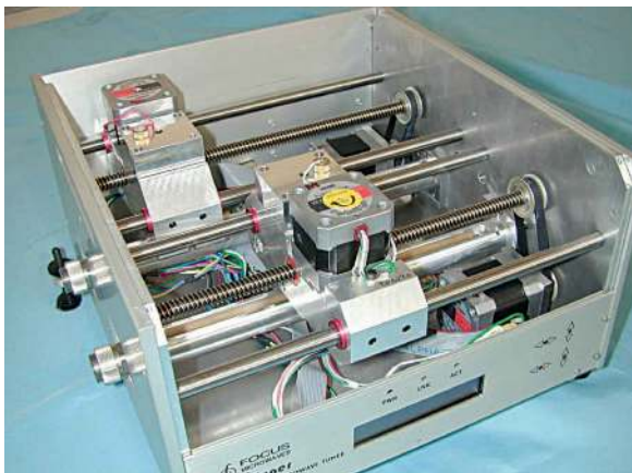
Figure 14. Differential tuner. (Photo courtesy of Focus Microwaves.)
