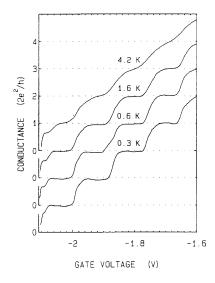
Figure 6. Conductance versus gate voltage at B = 0 and different temperatures. Increasing the temperature thermally averages the higher plateaus first (from Ref. [9]).
