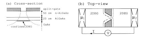
Figure 4. (a) Cross-section of a GaAs/AlGaAs heterostructure with typical layer thicknesses. A negative voltage  $V_{\rm G}$  applied to the metal split-gate confines the electrons laterally in the 2DEG.
