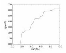
Figure 24. The dc current in nonlinear response versus  $eV = e(V_{\rm L} - V_{\rm R})$ , with  $V_{\rm L} = -V_{\rm R} = V/2$  and  $C_{\rm G}V_{\rm G}/e = 1$  fixed, for two doubly degenerate levels with  $\bar{\epsilon}_1 = 0$ ,  $\bar{\epsilon}_2 = 50$ , . The other parameters are T = 5, ,  $E_{\rm C} = 75$ , and ,  $^{\rm L} = , ^{\rm R} = , /2$ . All one-particle excitations of the dot are visible.
