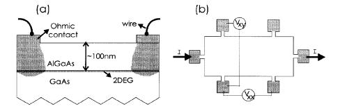
Figure 1. (a) Schematic cross section of a GaAs/AlGaAs heterostructure. The 2DEG is located at the interface between the GaAs substrate and the AlGaAs top layer. (b) Hall bar with six Ohmic contacts (shaded squares).
