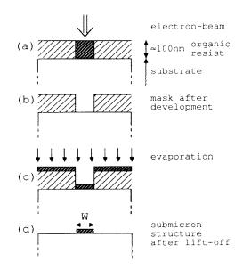
Figure 3. Outline of the electron-beam lithography procedure for fabricating submicron structures.
