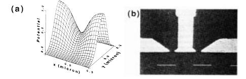
Figure 5. (a) Saddle-shaped potential induced in the 2DEG upon application of a negative gate voltage, resulting in lateral confinement in the x-direction and a potential barrier in the longitudinal y-direction (from Beenakker, and van Houten in Ref. [6]). (b) Scanning electron micrograph of a double-QPC device. The white areas are the Au gates, and the marker is 1  $\mu$ m long. The QPCs are 250 nm wide and are separated by 1.5  $\mu$ m.
