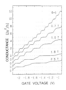
Figure 9. QPC conductance versus gate voltage at 0.6 K for several values of magnetic field. The increasing width of the plateaus demonstrate the increasing energy splitting in a magnetic field. The curves have been offset for clarity (from Ref. [18]).
