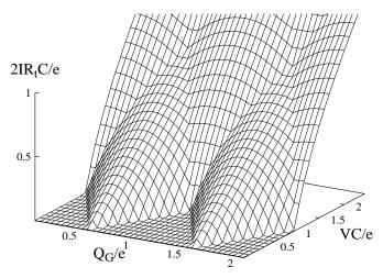
Figure 20. The current of a symmetric transistor is shown as a function of gate and transport voltage. At low temperatures and low transport voltages VC/e < 1 only two charge states play a role, and the Coulomb oscillations are clearly demonstrated. At larger transport voltages more charge states are involved.
