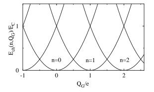
Figure 16. The charging energy of a single-electron box as a function of the gate voltage for different numbers n of electron charges on the island.
