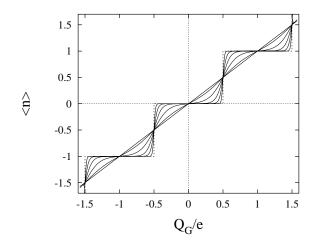
Figure 17. The average number of electron charges  $\langle n \rangle$  on the island of a single-electron box as a function of the gate charge (voltage) for different temperatures  $T/E_{\rm C} = 0$  (dashed steps), 0.02, 0.05, 0.1, 0.2, 0.4, and 1 (nearly linear).
