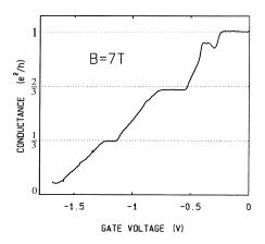
Figure 13. Two-terminal conductance of a quantum point contact at B = 7T. At zero gate voltage the conductance is  $G = e^2/h$  implying that the 2DEG is spin-polarized at filling factor 1. On decreasing the gate voltage fractional plateaus are observed (from Ref. [37].
