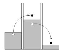
Figure 22. In an inelastic cotunneling process two electrons tunnel coherently, i.e. in a single qutnum process, in the left and right junction. The result is the transfer of charge through the system even in the Coulomb blockade regime. A particle-hole excitation is left in the island.
