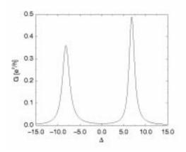
*Figure 25.* The differential conductance as a function of  $\Delta = \bar{\epsilon}$  for a two-fold degenerate level with large charging energy  $E_{\rm C}$  so that double occupancy can be neglected. T = 0.25,  $\mu_{\rm L} = -\mu_{\rm R} = 15$ , and  $L^{-1} = R^{-1} = R^{-1} = R^{-1} = R^{-1}$ .
