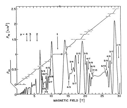
Figure 2. Measurement of the Hall resistance  $R_{xy}$  and the longitudinal resistance  $R_{xx}$  at 0.1 K. The mobility is  $\mu = 1.5 \cdot 10^6 \text{ cm}^2/\text{Vs}$ , the temperature is T = 80 mK. (Figure provided by R. L. Willett.)
