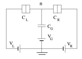
Figure 18. The SET transistor.
