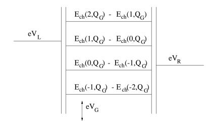
Figure 19. In the island the energy differences corresponding to the addition or removal of an electron charge are shown. They can be shifted by the gate voltage  $V_{\rm G}$ . The electrochemical potentials of the leads are shifted relative to each other by the transport voltage  $V = V_{\rm L} - V_{\rm R}$ .
