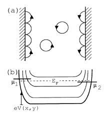
Figure 10. (a) Schematic classical electron trajectories in a magnetic field. (b) Corresponding quantum picture of the energy states of Eq. (10) along a cross-section of the 2DEG, illustrating the formation of edge channels at the boundary of the 2DEG (formed by the electrostatic potential energy eV(x, y)) where the Landau levels intersect the Fermi energy  $E_{\rm F}$ .
