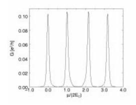
Figure 23. Linear conductance versus  $\mu$  for two doubly degenerate levels with  $\bar{\epsilon}_1 = 0$ ,  $\bar{\epsilon}_2 = 25$ , T = 5,  $E_C = 75$ , and L = , R = , /2. The distance between the second and third main resonance is larger due to the finite level spacing. All resonances involving excited states are hidden.
