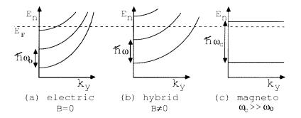
Figure 8. 1D subband dispersion for three values of the magnetic field, illustrating magnetic depopulation. The energy splitting is electric  $(\hbar\omega_0)$  in (a), and hybrid  $(\hbar\omega, with \omega^2 = \omega_0^2 + \omega_c^2)$  in (b). For large magnetic fields (c) the 1D subbands are Landau levels with an energy splitting of  $\hbar\omega_c$ .
