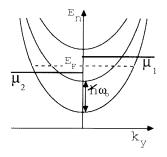
Figure 7. Energy  $E_n$  versus longitudinal wave-vector  $k_y$  from Eq. 4 at the bottleneck of a QPC assuming a parabolic confinement potential. The 1D subbands are separated by  $\hbar\omega_0$ . A net current results from the uncompensated occupied electron states in the interval between  $\mu_1$  and  $\mu_2$ , the electrochemical potentials of the two wide 2DEG reservoirs.
