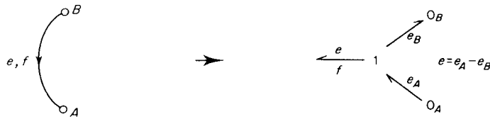
Figure 8.35. A linear graph line segment and its nodal bond graph equivalent.
