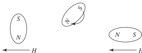
Figure 1.18 Effect on a magnetic dipole of a magnetic field H applied in the direction normal to polarization.
