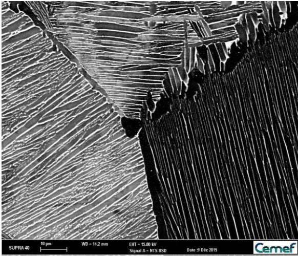
Figure 2. An initial microstructure of TA6V, with 3 different colonies.
