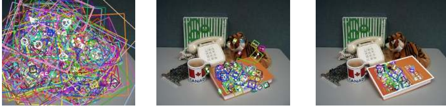
Figure 4: Finding consistent sets of feature matches. To find inliers to a homography we use a Hough transform followed by RANSAC. In this example, the test image was 640 \times 512 pixels. The number of initial matches to consider was 5469, which was reduced to 279 by broad-bin Hough transform clustering, and further to 104 matches in the final solution using RANSAC.
