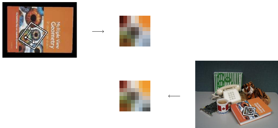
Figure 3: Extraction of affine invariant features from a pair of images. Groups of 3 interest points are used to calibrate the affine transformation to a canonical frame. The image region is then resampled in the canonical frame to form the feature descriptor.
