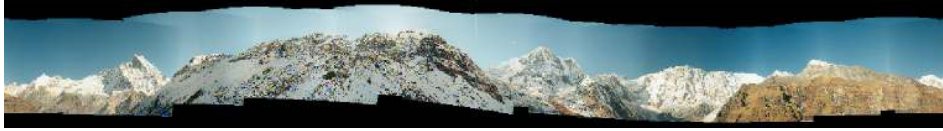
Figure 7: Cylindrical panorama of the Annapurna sequence of images. This was computed by estimating the (3 dof) rotations between images from feature matches.
