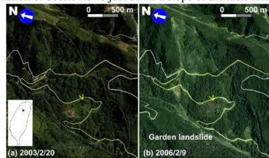
Figure 11. The remote sensing images of Garden Landslide before and after disaster (white dashed line is the landslide boundary; base map is from Google Earth)
