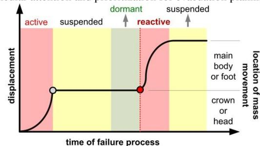
Figure 14. Displacement as a function of the failure process. Reactivation after suspension indicates a renewal of dormant deep-seated landslides (modified from Cruden and Varnes, 1996)
