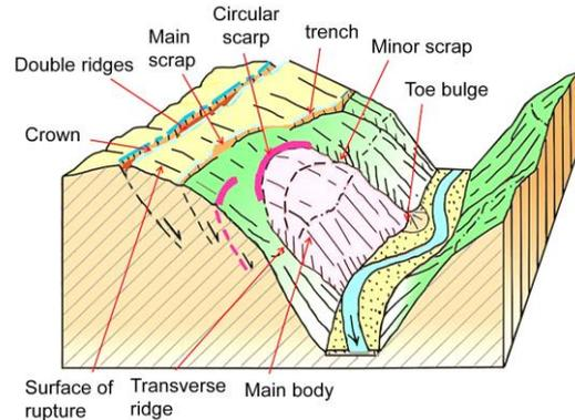
Figure 4. deep-seated landslide characteristics (modified from Takasuke, 2000)
