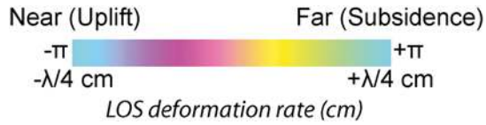
Figure 2. The difference in deformation rate between places having the same color is a multiple of \lambda/2 . When the color turns from pink to yellow, the ground moves far from the satellite. In the opposite direction, the ground moves near the satellite.
