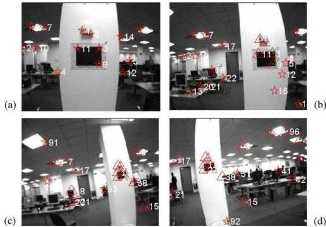
Fig. 15. Parametrization switching seen in image space: points coded in inverse depth ( \star ) and coded in XYZ ( \triangle ). (a) First frame, with all features in inverse depth. (b) Frame #100; nearby features start switching. (c) Frame #470, loop closing; most features in XYZ. (d) Last image of the sequence.
