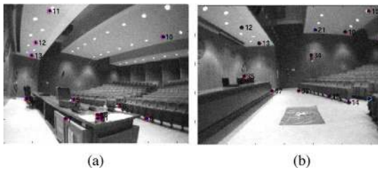
Fig. 6. First (a) and last (b) frame in the sequence of the indoor experiment of Section VII-A. Features 11, 12, and 13 are analyzed. These features are initialized in the same frame but are located at different distances from the camera.
