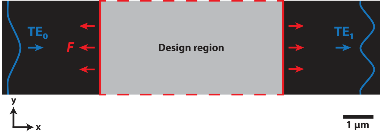
Figure 3: Design setup for the optimization of a waveguide mode converter. The design region (dashed red rectangle) has an area of 4\ \mu\text{m} \times 6\ \mu\text{m} and is embedded in a waveguide ( n = 1.5 ) with a width of 3\ \mu\text{m} surrounded by air ( n = 1 ). The fundamental \text{TE}_0 mode with an operating wavelength of 1\ \mu\text{m} is injected into the waveguide from the left. The electromagnetic design goal is the maximization of the mode overlap with the second order \text{TE}_1 mode at the right end of the waveguide. The structural problem is defined as the compliance minimization of the material ( Y_{\text{max}} = 1 ) within the design region with respect to two opposing forces placed at its left and right edges.
