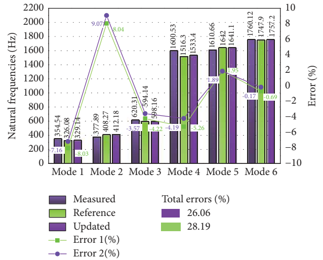
FIGURE 9: Comparisons of natural frequencies from the test (measured), the analytical model (reference), and the updated FE model (updated) at a pretightening torque of 30 N·m.
