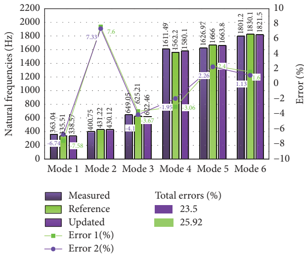
FIGURE 12: Comparisons of natural frequencies from the test (measured), the analytical model (reference) and the updated FE model (updated) at a pretightening torque of 60 N·m.
