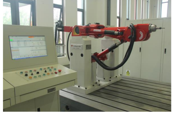
Fig. 11. A prototype machine of the TriMule robot
