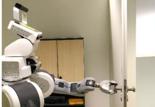
Figure 1. This picture shows the door opening task that we use to evaluate our approach by first learning a cost function from demonstration and then generating motions by optimizing the cost function for different scenarios (e.g., initial positions, door angles). See Section 6.5 for more details.
