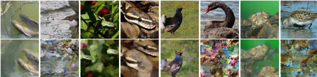
Figure 3: Single-Image Reconstruction from the parameter gradients of trained ResNet-152. Top row: Ground Truth. Bottom row: Reconstruction. We check every 1000th image of the ILSVRC2012 validation set. The amount of information leaked per image is highly dependent on image content - while some examples like the two tenches are highly compromised, the black swan (ironically) leaks almost no usable information. Noticeable is also the loss of positional information in several images.
