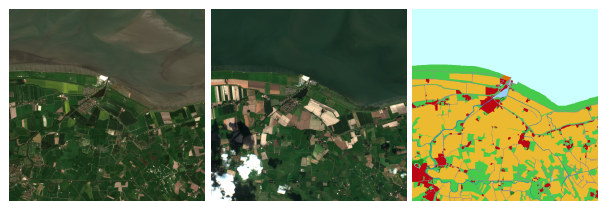
Figure 3. A Sentinel-2 tile of size 8 \times 8 \text{ km}^2 for April 2019 (left), September 2020 (middle), and the corrected reference for 2020 (right). The colours correspond to: red - bld. , grey - sld. , yellow - agr. , light green - grl. , dark green - for. , dark blue - fwt. , light blue - swt. , turquoise - sea , brown - bar.
