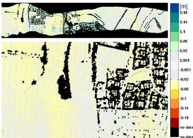
Figure 7: Strip differences for the improved georeferencing after the strip adjustment; cf. fig. 6. Note that the systematic patterns of the height differences, which are visible in fig. 6 (especially at the roofs), have now disappeared to a very high degree.
