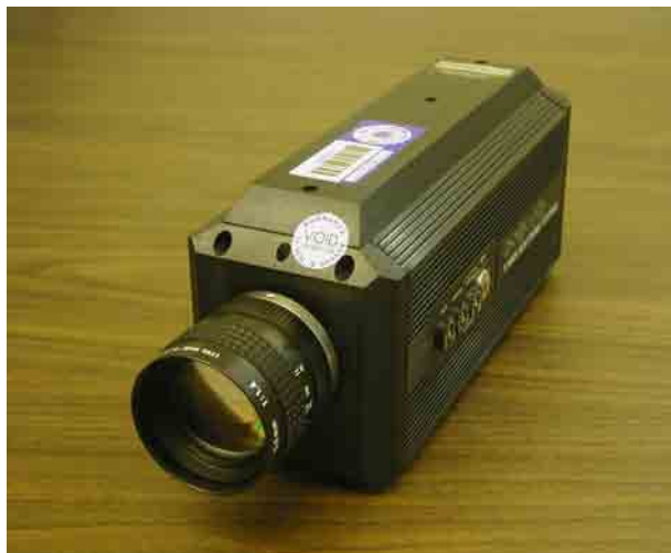
Figure 3.4. Xybion ISG – 780 Intensified CCD camera.
