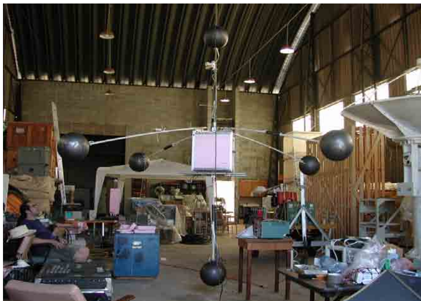
Figure 3.2. University of Washington balloon payload, under testing in INPE hangar at Cachoeira Paulista.
