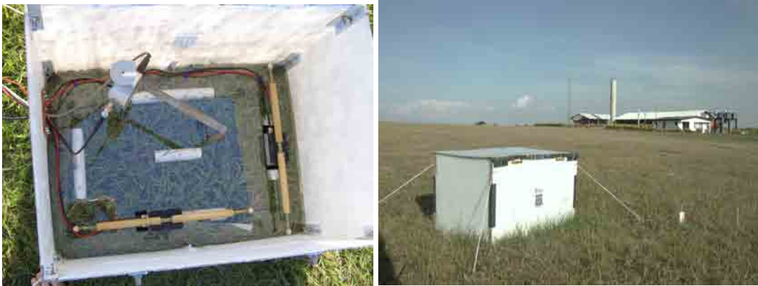
Figure 4.7. (a) Duke University electromagnetic sensors, used to measure lightning sferics, and (b) system deployment at SSO.
