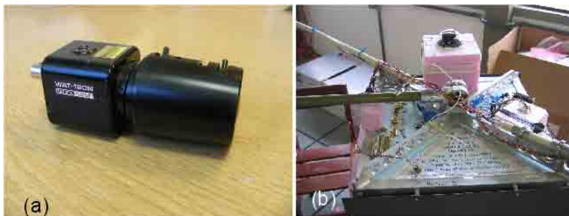
Figure 4.3. (a) WATEC 120N Camera, fitted with a Fujinon all-sky (180°) lens. (b) Close-up showing WATEC camera mounted on top of the balloon payload (in pink insulated box).
