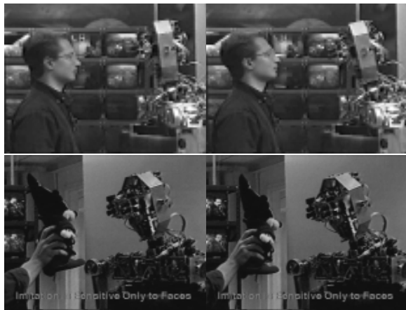
Figure 12: Images captured from a videotape of the robot imitating head nods. The upper two images show the robot imitating head nods from a human caretaker. The output of the face detector is used to drive fixed yes/no nodding responses in the robot. The face detector also picks out the face from stuffed animals, and will also mimic their actions. The original video clips are available at http://www.ai.mit.edu/projects/cog/ .
