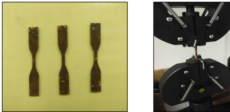
FIGURE 1 Type V Dog Bone Specimen used for Tensile Testing
