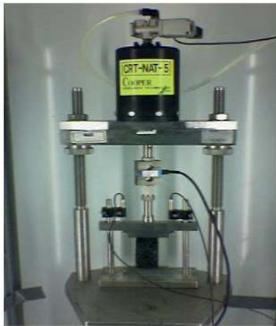
Fig. 2 Samples loading in the fatigue test
