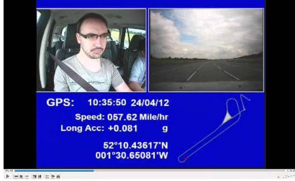
Figure 8: Screen shot of the video recorded during the trials, with driver and forward facing cameras, as well as GPS details overlaid.
