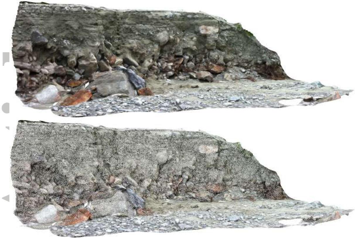
Figure 3: Examples of image-covered polygonal mesh (above) and its wireframe (below), generated using Iphone 4 images and 123D Catch.
