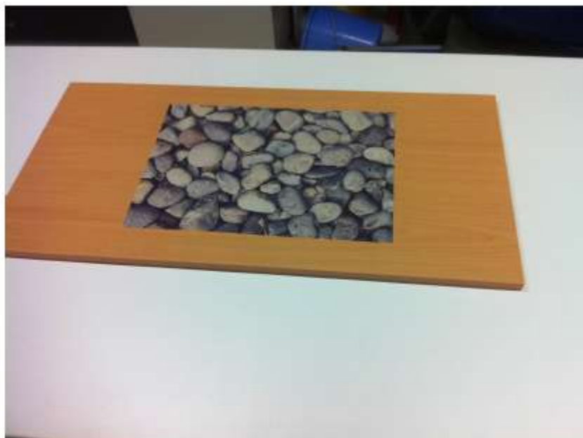
Figure 7: Set up for the experiment: high quality print pasted on a wooded plank to be as at as possible.
