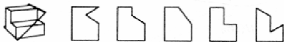
Figure 1: Test of mental transformation, the Mental Cutting Test, consisting of 25 items in 20 minutes - identify the cross section after the following transformation has occurred (answer: second from right)
