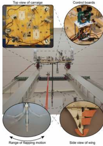
Figure 3: Carriage setup highlighting the pulley system setup, control boards, range of wing motion and wing structure.
