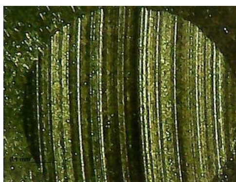
Fig. 8. Contact area of samples after four-ball machine test in Litol-24.
