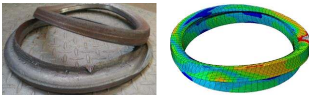
Figure 8. Final geometries in case, the inner ring grows too fast and outgrows the outer ring. left : rolling experiment right : FEM-simulation.
