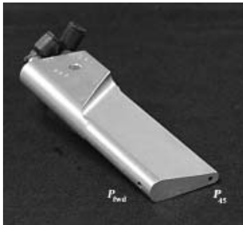
Figure 2. Pressure port locations.
