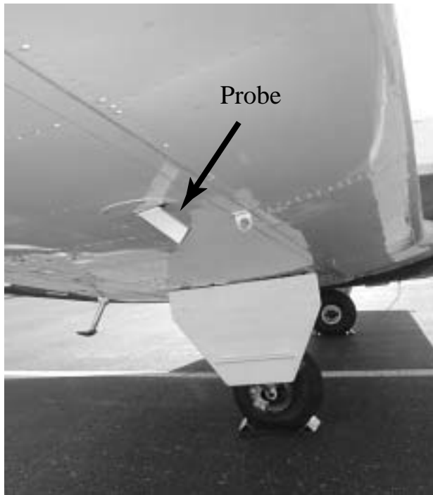
Figure 1. Angle of attack probe mounted under the wing.
