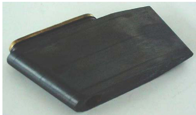
Fig. 4. Simple hydrofoil with a swept leading edge.
