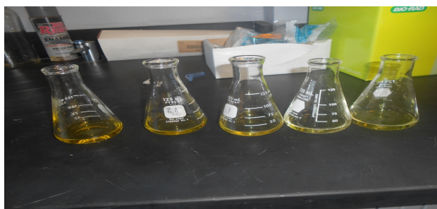
Figure 1. Acid (HCl or CH 3 COOH) solution plus three drops of natural indicator (waakye leaves extract). Color change was yellow.
