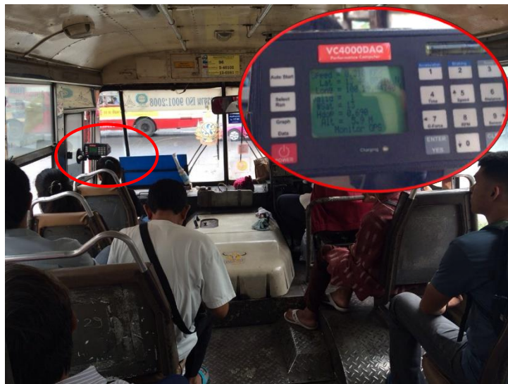
Figure 3. Kinematic measurement of public bus using VC4000.
