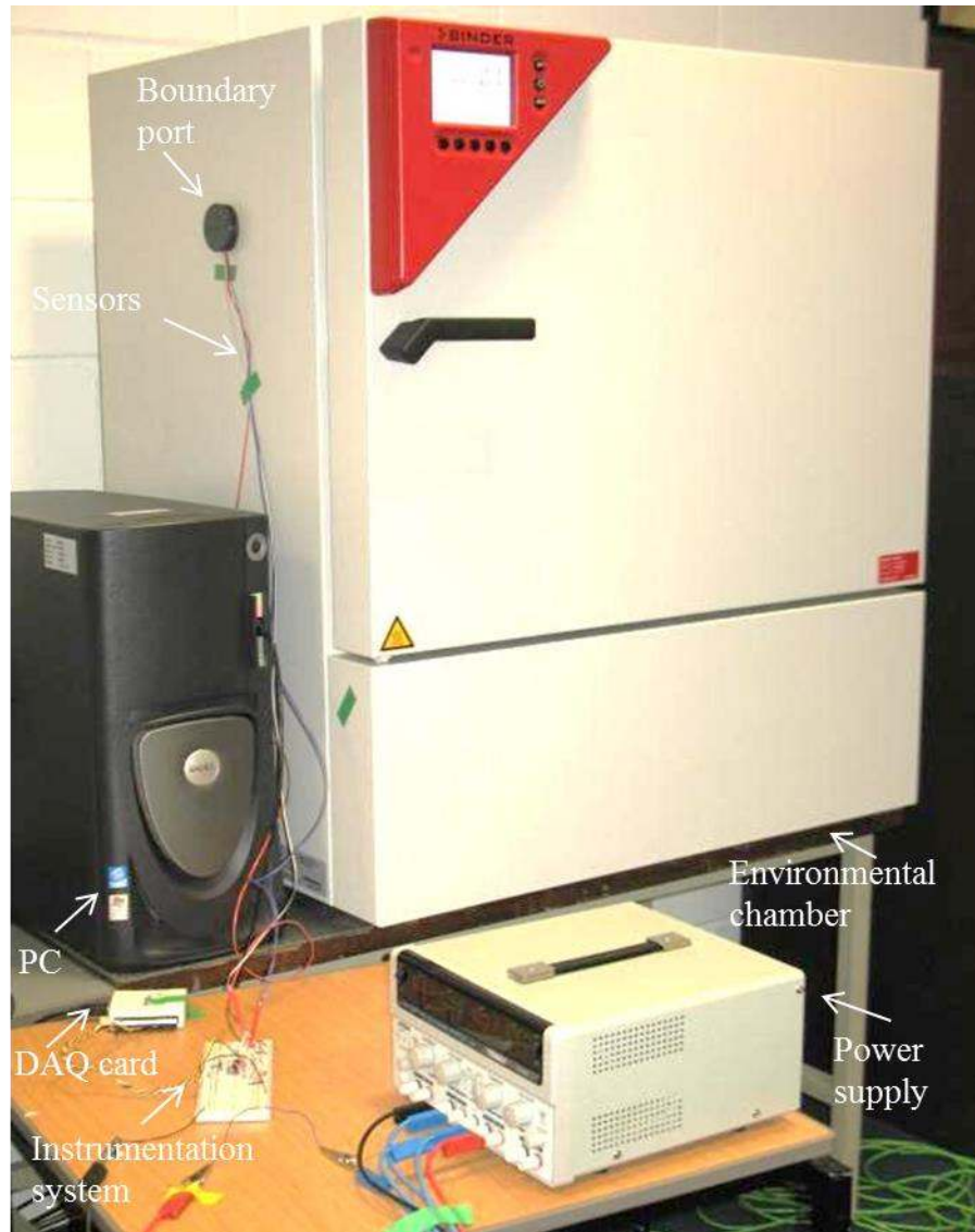
Figure 7.8: Exterior of the advanced T-history setup.
