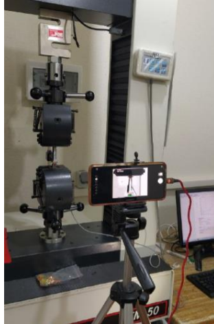
Fig 2. Machine setup for the tensile test(29).
