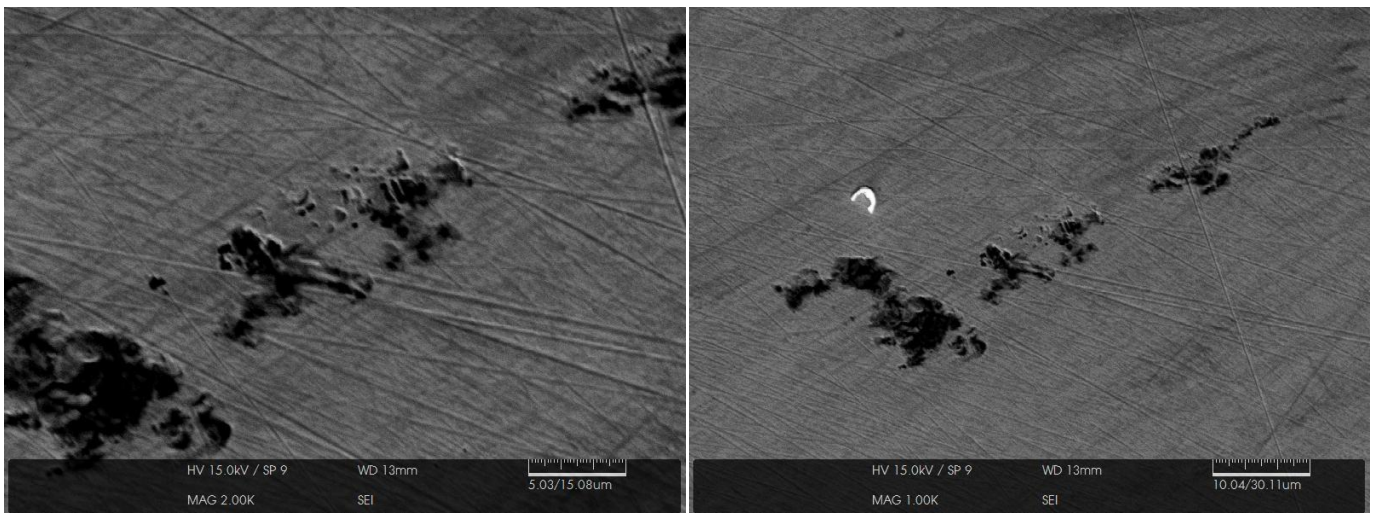
Figure 5: SEM morphologies of certain region of welded coupon sample with 2 nd cyclic heat treatment (Set C) after Pitting Corrosion Test.
