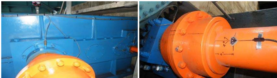
Figure 97. Instrumentation of the mechanical parts: accelerometers at the gearbox and strain rosettes at the drive shaft
