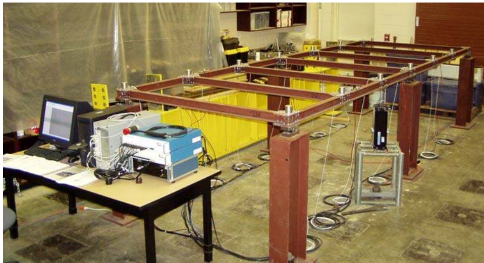
Figure 8. The steel grid model used for the experimental studies
