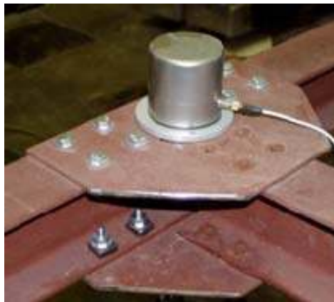
Figure 12. Removal of the bolts at N3 and N10 for DC1
