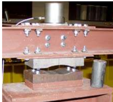
Figure 14. Removal of the roller support at N4 for DC3
