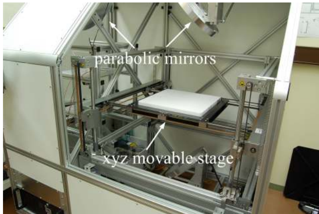
Figure 1. Photograph of the mmW focusing system.
