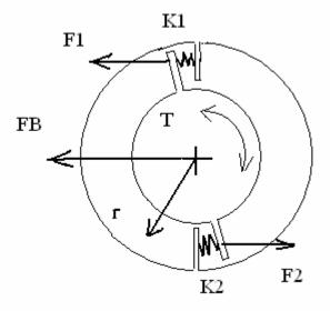
Figure 5 Equivalent dynamic model of flexible coupling.
