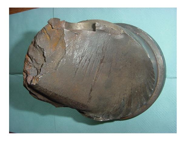
Figure 1 View of fractured shaft looking from coupling end towards generator.
