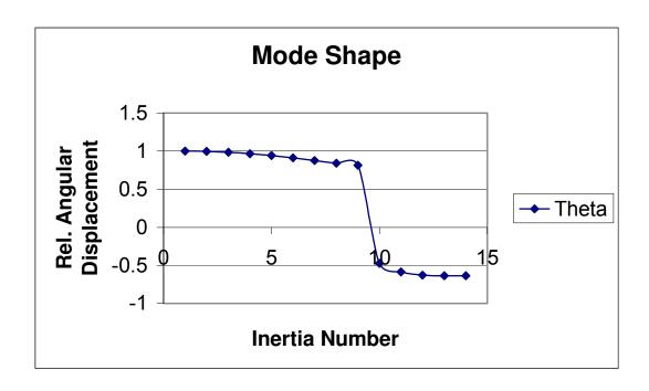
Figure 7 Torsional mode shape for diesel-generator at 89% load.
