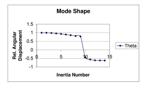
Figure 6 Torsional mode shape for diesel-generator set at full load.
