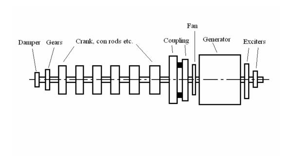
Figure 4 Schematic diagram of diesel-generator system.
