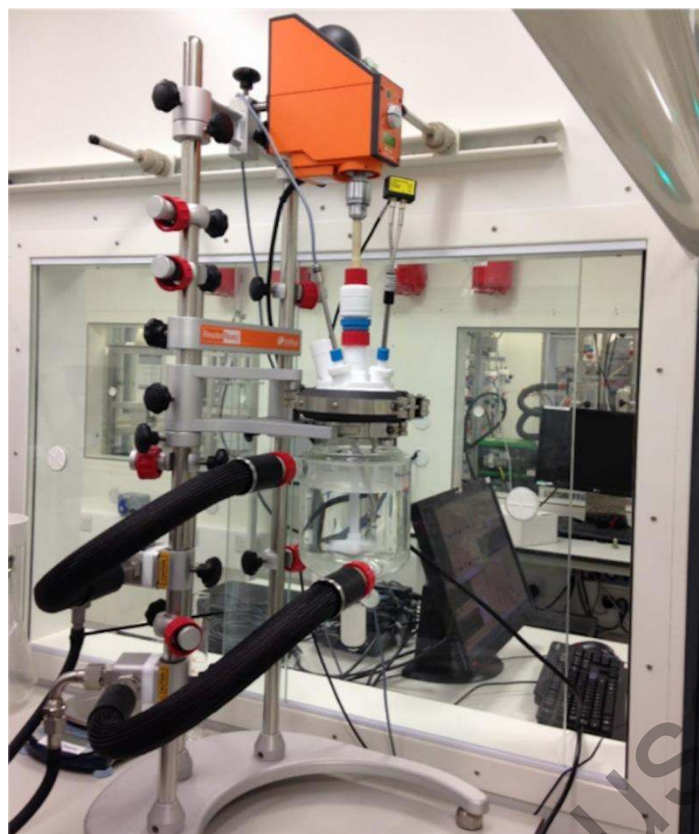
Figure 3 Set up of stirred tank vessel for dissolution experiments
