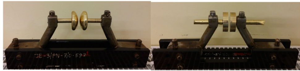
Figure 2. Electrode holder assemblies (left—VDE, right—disc electrode).
