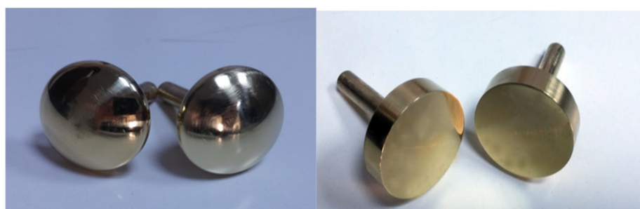
Figure 1. VDE (left) and disc (right) electrodes used in experiment.
