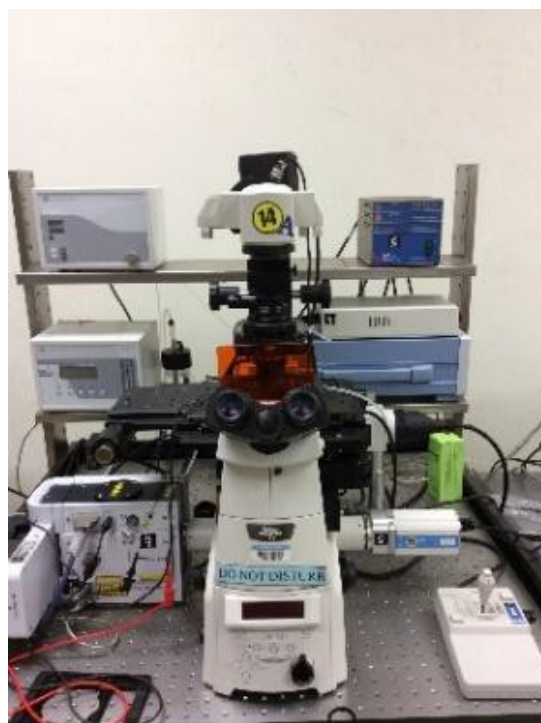
Fig. 3(a-c): (a) High voltage pulsed system (ECM® 830), (b) Chamlide TC stage and (c) Microchamber slide (Chamlide EC)
