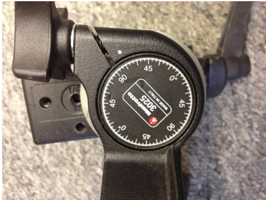
Figure 3.6 A scale was provided on every camera's mount to help with recording camera's rotation angle.
