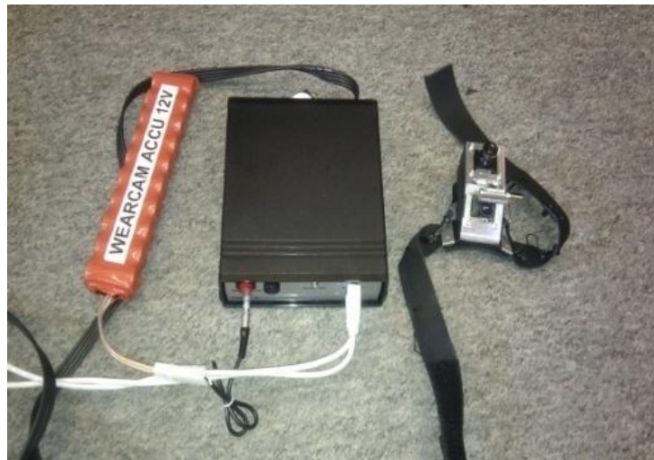
Figure 5.1 The Wear Cam eye-tracking equipment is shown, including rechargeable batteries (left), connector box with USB cables (middle) for PC input, and cameras mounted on the headband worn by the subject.
