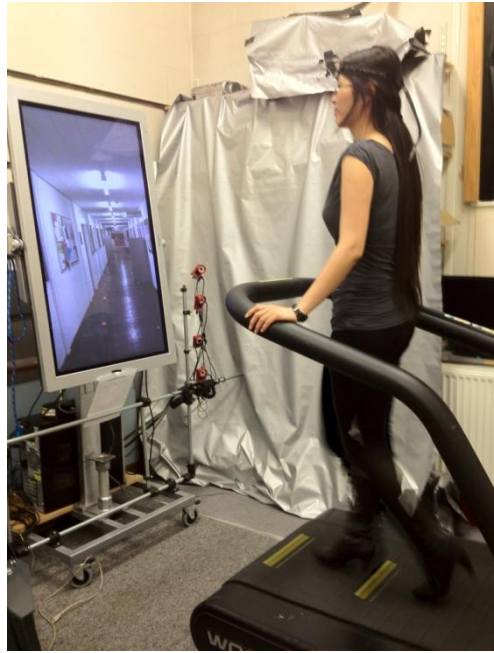
Figure 5.4 Subject walks on the StroMoHab locomotion simulator while wearing the eye-tracker, as the simulated video environment is played in the screen. In this simulated environment, subjects were provided with normal indoor lighting conditions, while avoiding reflections on the screen.
