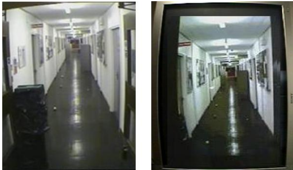
Figure 5.5 A photograph to illustrate the matched visual angles in the RE (left) and SE (right) within the scene of the corridor path. The visual angles of target objects were equal in the two environments, although the full field of view in SE was narrower in both height and width in comparison to the RE. Regions outside the SE view did not contain target objects for the SAC task. Note that any geometric distortions in this figure are due to capturing the image and were not present in experiments for this figure.
