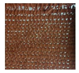
Figure 8. Iron oxide-coated sisal fiber-based filter media.
