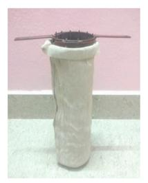
Figure 3. Zinc oxide-coated sisal fiber-based filter media.
