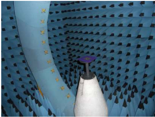
FIGURE 10: Antenna's measurement setup in Satimo stargate SG 32 anechoic chamber.
